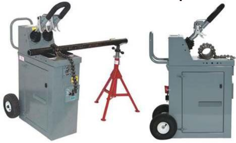
The Kwik-Snap<sup>™</sup> 2500 Production Cast Iron Soil Pipe Cutter is a powerful portable high volume soil pipe cutter for cast iron pipe. With its 3.5 second cutting cycle time from the electric hydraulic power, you can cut more pipe faster to get the job done quickly. It has a capacity of 1-1/2" to 6.00" OD pipe and its unique chain design cuts pipe fast, thus eliminating the need to reset for each cut on the same size pipe. It is quiet and reliable and easy to use.
